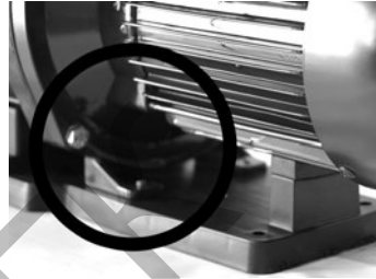
Regularly check the waterproofness! (A leak through a mechanical seal can cause important damages!)
