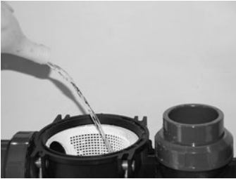
Prime the pump (if not risk of dry running). WARNING! RISK OF DRY RUNNING!!
